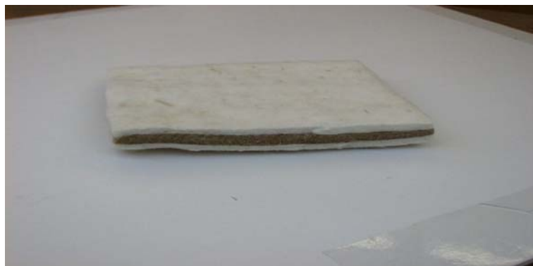
Figure 1-22. Three Layer (sandwich type) Nonwoven Composite – Ramie/Kenaf/Polypropylene
