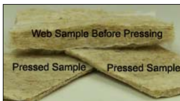
Figure 4-1. Layered composite nonwovens made of bagasse/cotton webs and EBC melt blown nonwovens before and after hot-pressing.
