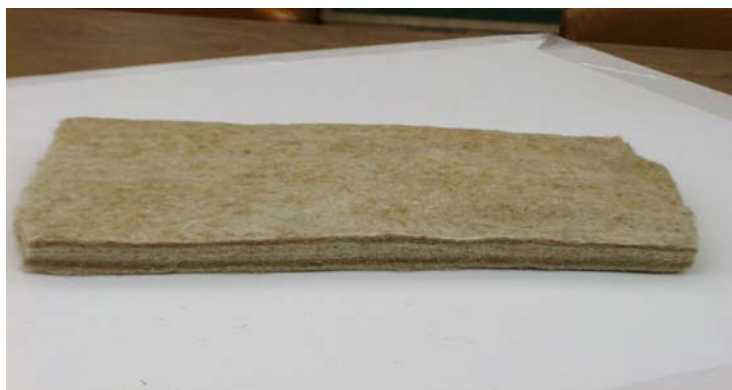
Figure 1-23. Three Layer (sandwich type) Nonwoven Composite – Bagasse/Kenaf/Polypropylene
